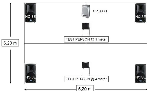
Figure 1. Schematic lay-out of the test set-up. The height of the room was 2.60 meters.
